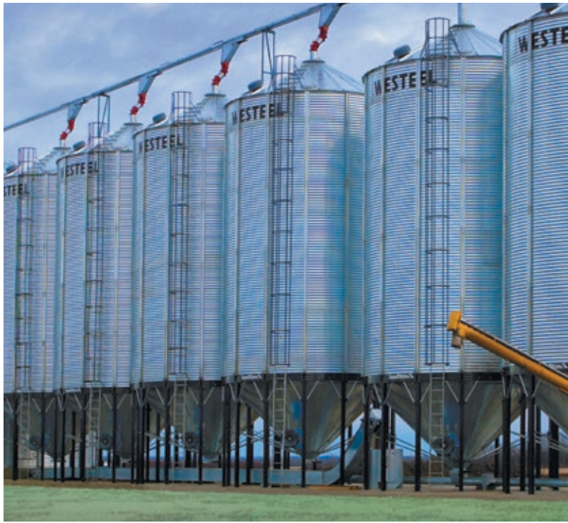
A All SSK models now feature a more efficient ring beam B Controlled from ground level, the remote cap opener opens in a horizontal sliding motion to avoid wind damage (the 33" fill cap opening mechanism is protected from the elements when the lid is closed) C Grain Gauge™ D Bolt-on inspection hatch E Pass through rail (optional) F Safety cage (optional)
