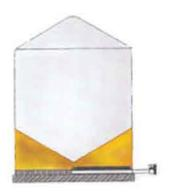
70 – 80% of the grain is removed through the center sump by gravity
