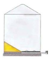
When the center sump runs empty, grain is removed through the intermediate sump(s) to free the sweep.
