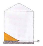
The sweep removes the remaining 20-30% of the grain.
